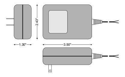
Power Supply for use with Ring-Master Intercom Systems. UL Listed and CE Marking Compliance. This power Supply is used for local Power of 900 type stations or to Power up to 5 Pro700 stations.
