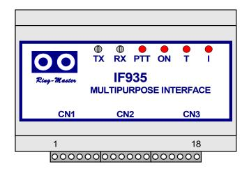
The IF935 Interface is used with CB901, CB901EX, RM5000 and RM5000EX central exchanges. The Interface provides 4 wire audio and control contact closures to external equipment. The audio is transformer coupled. Contact closures in the IF935 are galvanic isolated. Each IF935 require one subscriber position in the central exchange.
