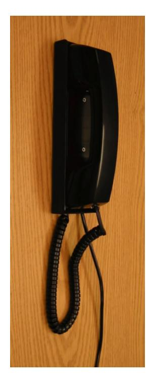
The GD591 handset assembly may be used with the AA903 and AA905 master-stations. The spiral cord for the K-style handset is standard 4 wire with modular connectors. A magnetic operated hook-switch design is used . The handset assembley is designed for surface wall mounting and a backbox is not needed.
